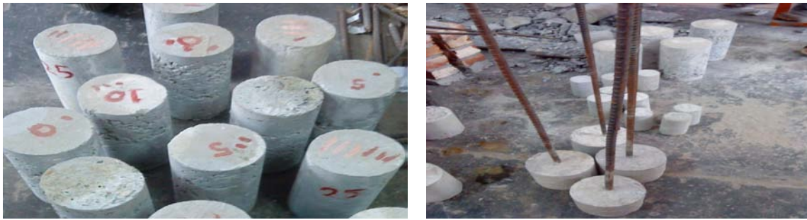
(a) (b) Figure 4: Cylinder for (a) Compressive Strength& (b) Bond Strength.
