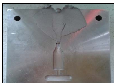
Fig.8 Incomplete molding of feedstock A70.
