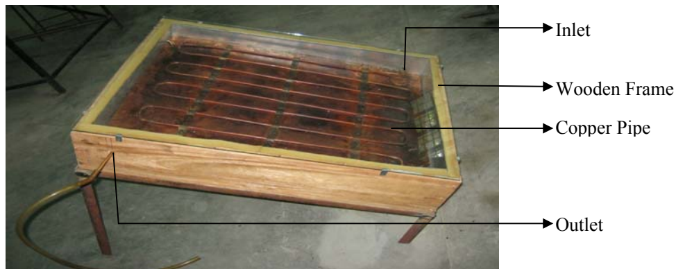
Fig.3 Photograph of our constructed solar collector
